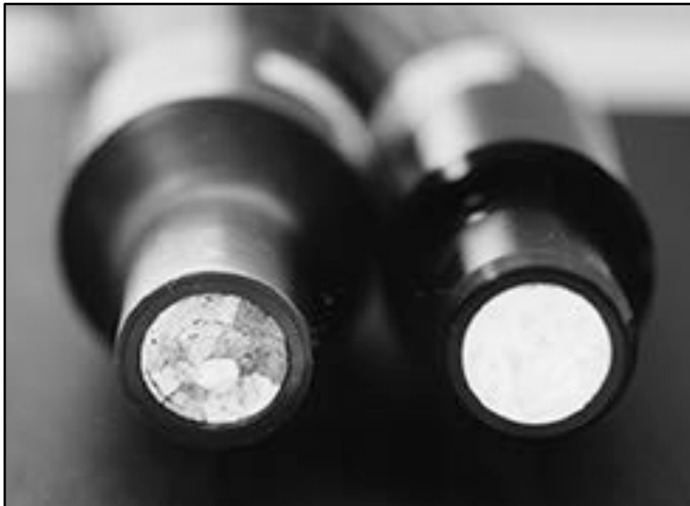
Figure B-10. On the left, a glass fiber common-end bushing, obscured. The lines and dark holes are the epoxy. On the right, a new unused bushing. The obscured end was removed from a museum installation after failure as a result of heat and intense light.
