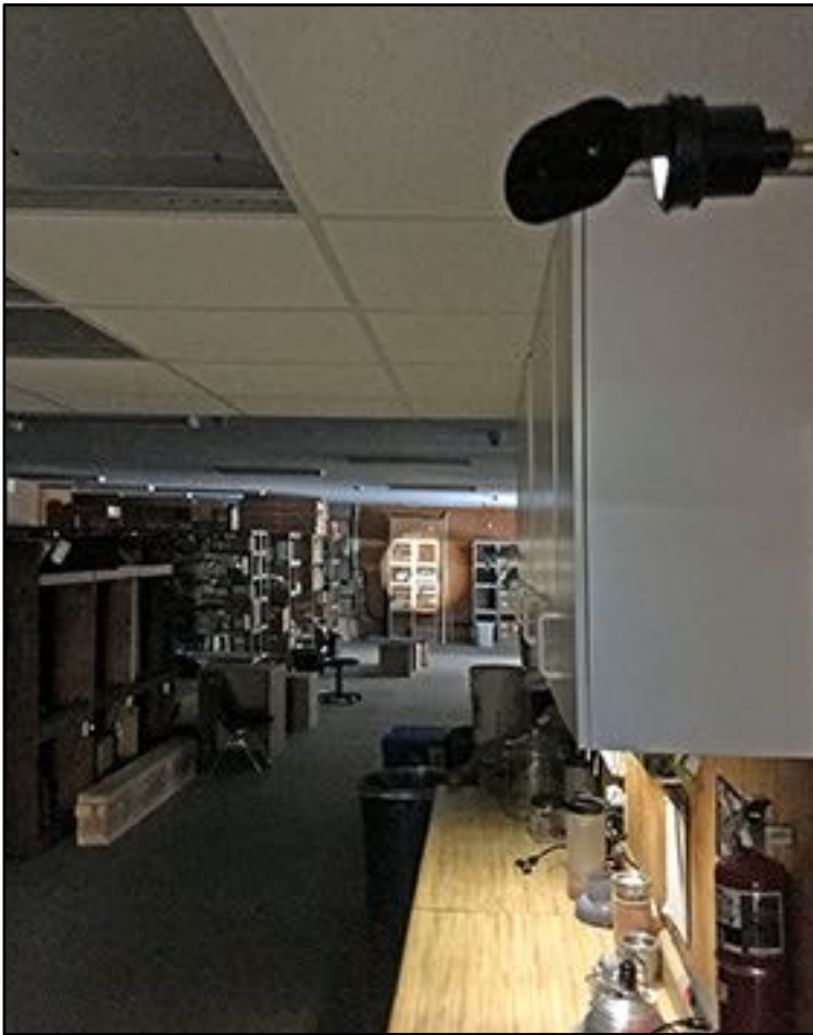
Figure B-16. A single pinspot powered by a single 3 mm acrylic fiber shines a beam from the outside wall of the lighting lab clear across and through the inventory stacks at the NoUVIR facility. This is over a 60-foot throw.
