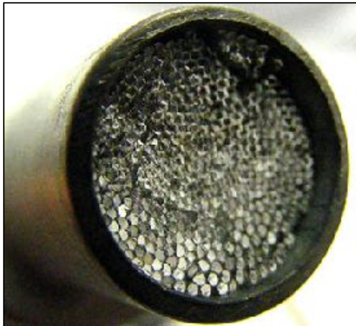
Figure B-3. Fused end of a fiber. Some of the strands are hex shape, yet others are overly melted.
