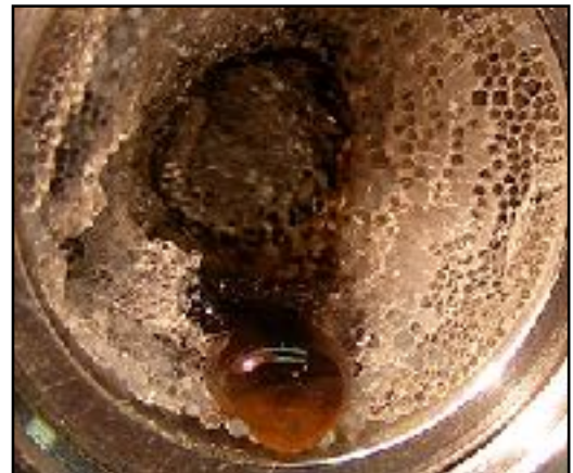
Figure B-7. A melted acrylic bushing found in a competitor's system that could no control heat build-up.
