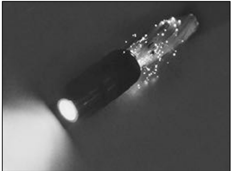
Figure B-8. Glass fiber breakage at 90° bend.
