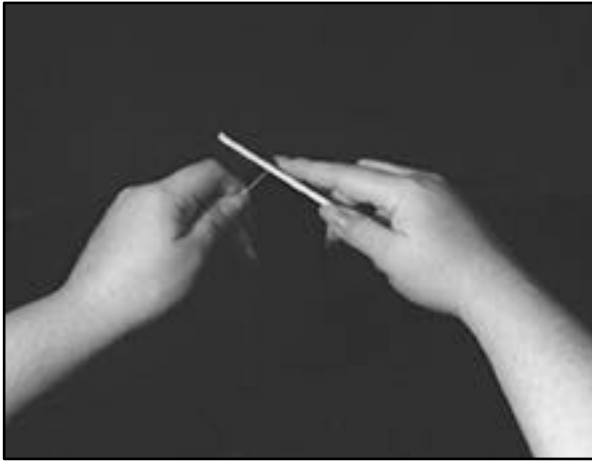
Figure B-15. Polishing solid pMMA acrylic fiber with a hand buff like those used on acrylic nails in a beauty salon.
