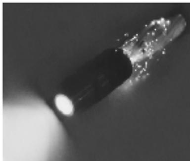
The jacketing is usually heavy enough that the breakage is not visible. This fiber simply got dimmer. It was not until it was cut into that the breakage was found where it bent into the luminaire. This means that in a visible fiber optic lighting system the way broken fibers are detected is by light loss.
