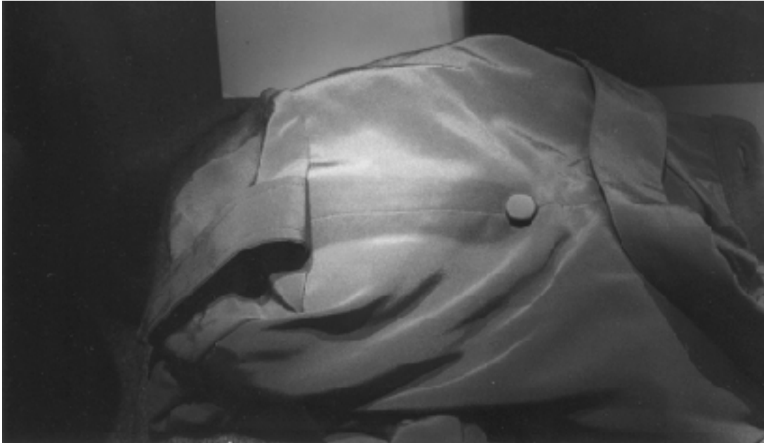
Figure 2-1. Detail of fading on silk dress after less than 30 days under fluorescent lighting.
