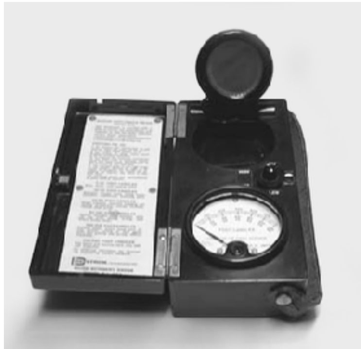
Figure 2-4. You can clearly see the dark CIE curve filter over the sensor head of this Weston light meter.
