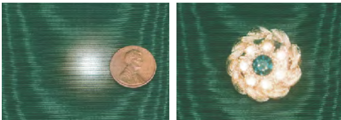
Figure 17. Control. Left - Beam of single “close-up” fiber optic luminaire shows control. Right - brooch with emerald lit at 300 fc, beams lighting diamonds to 100 fc and textile lit a 3 fc (REM filtered for green). Tight beam control can allow jewelry to be exhibited with costumes instead of in separate cases.
