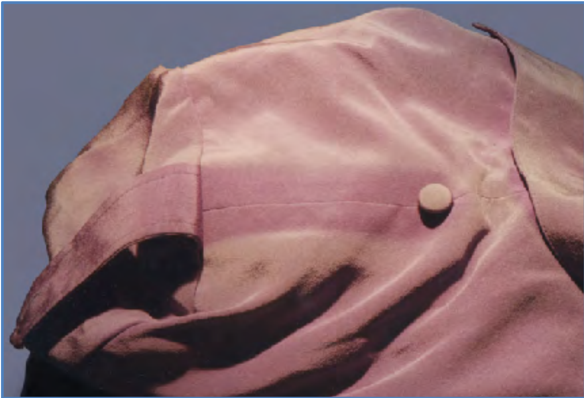
Figure 4. An example of fading due to UV, IR and color mismatched visible light.
