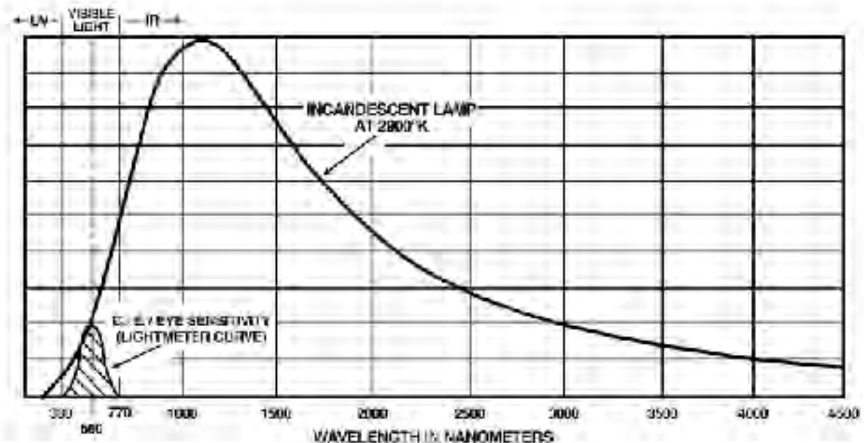
Figure 2 - Spectral output of a quartz-halogen lamp at 3200°K
