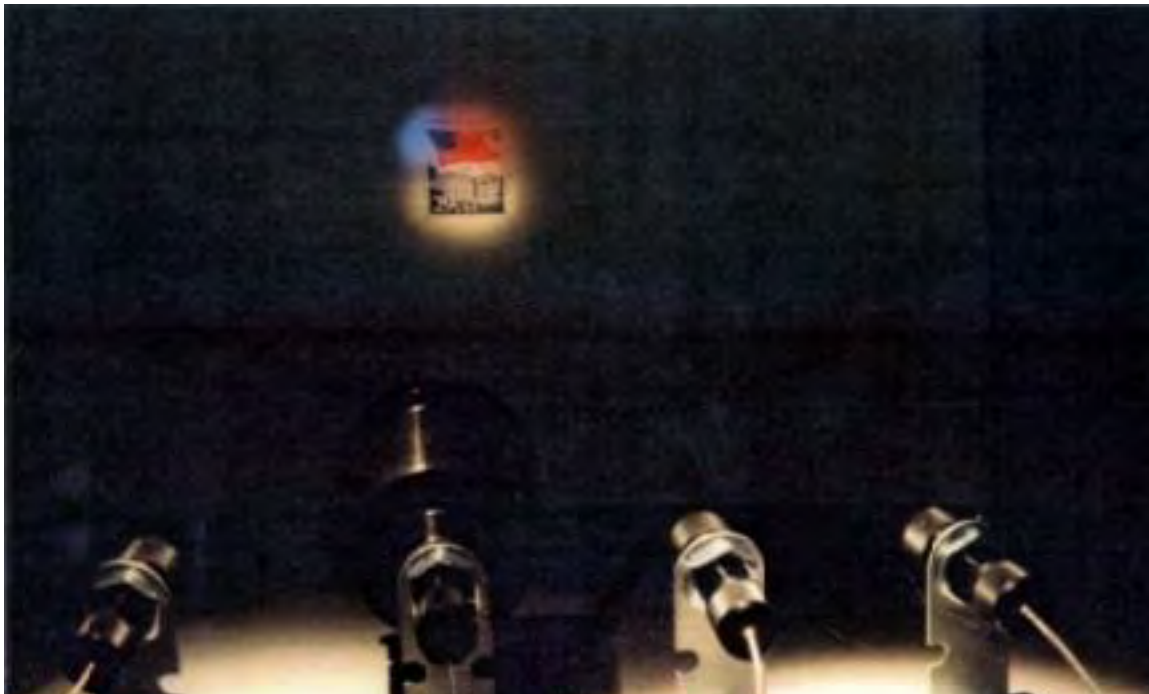
Figure 20. Application. Photograph intentionally shows bleed, so REM filters can be detected on 29¢ United States first class stamp.
