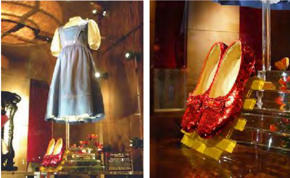
Figure 18. Application. Left - Rare Judi Garland “test dress”, 1 of 1, from the Wizard of Oz is lit at 16 fc from chest to hem. White blouse is embrittled and lit at 3 fc. Slippers at case’s floor are lit at 18 fc. Right - Ruby Red Slippers brilliantly sparkle.
