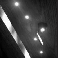
A polished bare fiber produces the same beam and intensity as a flood adjusted to its widest 72° beam. The difference is that without the luminaire body, aim is more difficult and there is no zoom control. In small enclosures or at close lighting distances, bare fiber can provide spectacular lighting at minimum cost. Several fibers with overlapping 72° beams give a wide, gentle wash.
