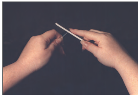
Now polish until it is clear and clean, insert the fiber into a luminaire and aim, focus, and light.
