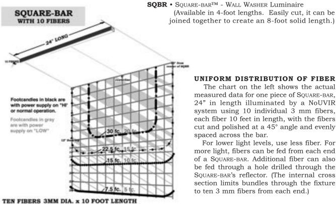
The chart on the left shows the actual measured data for one piece of SQUARE-BAR, 24" in length illuminated by a NoUVIR system using 10 individual 3 mm fibers, each fiber 10 feet in length, with the fibers cut and polished at a 45° angle and evenly spaced across the bar.
